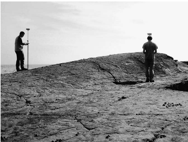
Fig. 1. Analysis of folded bedding surface at Howick, Northumberland, using RTK GPS. View looking south east.
